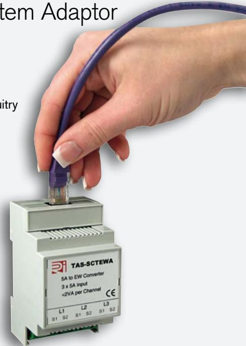
The **TAS-SCTEWA** converter allows for the connection of up to three standard current transformers, or standard split-core current transformers (with 1A or 5A secondary's), to the Rayleigh Instruments **easywire®** system.
